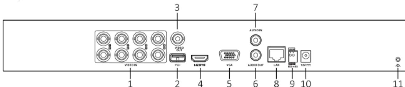
\*: The rear panel of iDS-7204HUHI-M2/S and iDS-7216HUHI-M2/S provide 4 or 16 video input interfaces.
